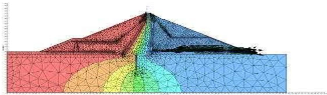
Figure 5: Flow network and seepage from dam
