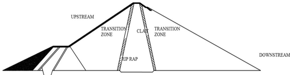
Figure 1: Cross Section of Duhok Dam
