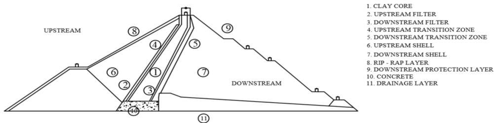
Figure 2: Cross Section of Ilam Dam
