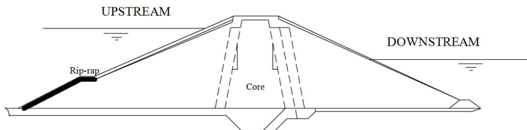
Figure 3: Cross section of Bar dam
